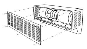
Figure 3 - Removing Air Intake Grille
